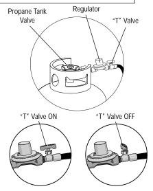
NOTE: Type 1 fittings are made with a metal to metal seal and must be made very tight to prevent leaking.
